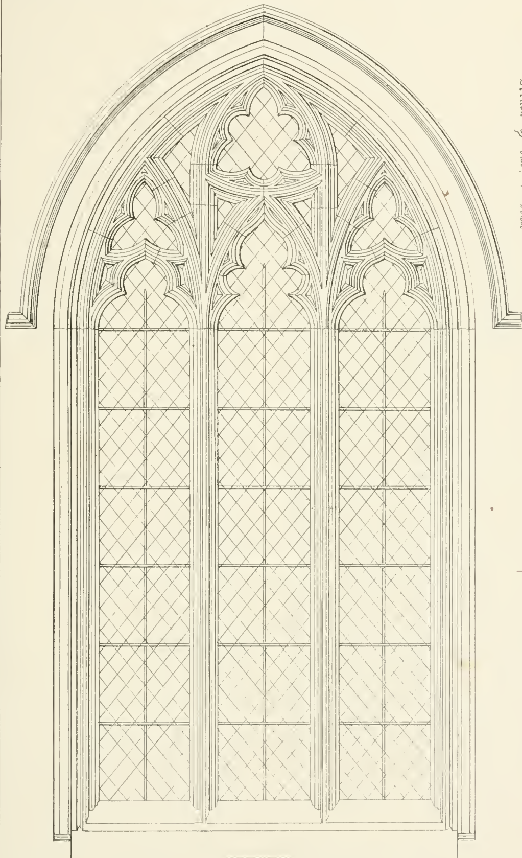
Window in North Aisle Bottisham Ch Cambridge Scale of 1 / 2 inch = 1 foot
